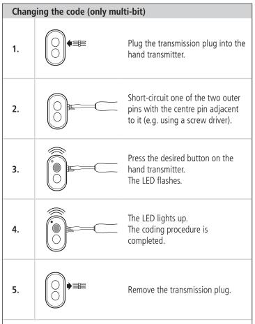
After the hand transmitter has been re-coded, the operator system must also be re-programmed to respond to the new code. For multi-channel transmitters, the programming process must be carried out for each button separately.
